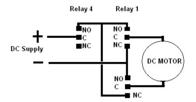
The left/right (CCW/CW) direction is the same circuit with relays 2 and 3.
