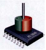
The AS5040 was produced to provide the radial location of steering wheels, accelerator pedals etc in fly by wire applications. The chip is capable of providing accurate readouts without missing a location on a shaft rotating at 600RPM. It is not anticipated that the capabilities of the chip will be stressed by beam rotation speeds! The chip samples each location at 12KHz.
