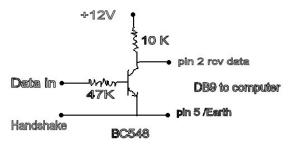
You will also need to put SW2 in the ON position (0V) and ground the handshaking line that normally goes to pin 7 of the DB9.
