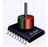
The AS5040 was produced to provide the radial location of steering wheels, accelerator pedals etc in fly by wire applications. The chip is capable of providing accurate readouts without missing a location on a shaft rotating at 600RPM. It is not anticipated that the capabilities of the chip will be stressed by beam rotation speeds! The chip samples each location at 12KHz.
