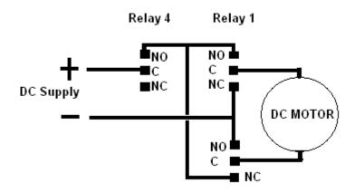
The left/right (CCW/CW) direction is the same circuit with relays 2 and 3.
